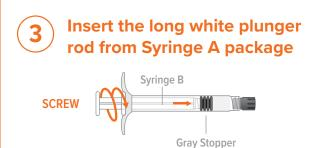
Gently screw the white plunger rod into the remaining gray stopper in Syringe B.
