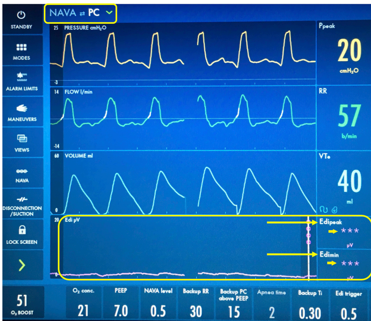
Figure 1. Invasive neurally adjusted ventilatory assist (NAVA) ventilator screen. No Edi peak or Edi minimum readings are recorded at this time, demonstrating no patient electrical signal with which the ventilatory system can synchronize. As a result, the ventilator pressure control backup is providing ventilator set rate breaths.
