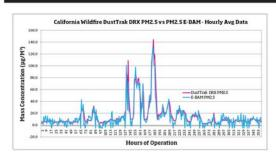
The PM2.5 24-hour average data from the DustTrak Environmental Monitor is shown to compare extremely well with the E-BAM (slope of 0.993 and R^2 of 0.99), as supported by the correlation plots above.
