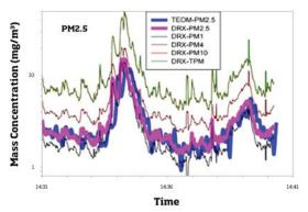
Comparison of Arizona Road Dust mass concentration measured by the DustTrak DRX and the TEOM with a PM2.5 impactor.
