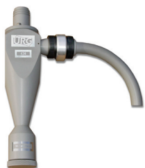
92Lpm 2.5µm Sharp Cut Cyclone
